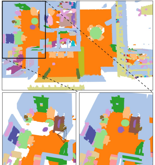
Figure 5. Language map incrementally created with our adaptive optimization. Bottom Left : A region mapped in the beginning. Bottom Right : The same region after the mapping is completed. All initially mapped objects remain unchanged.
