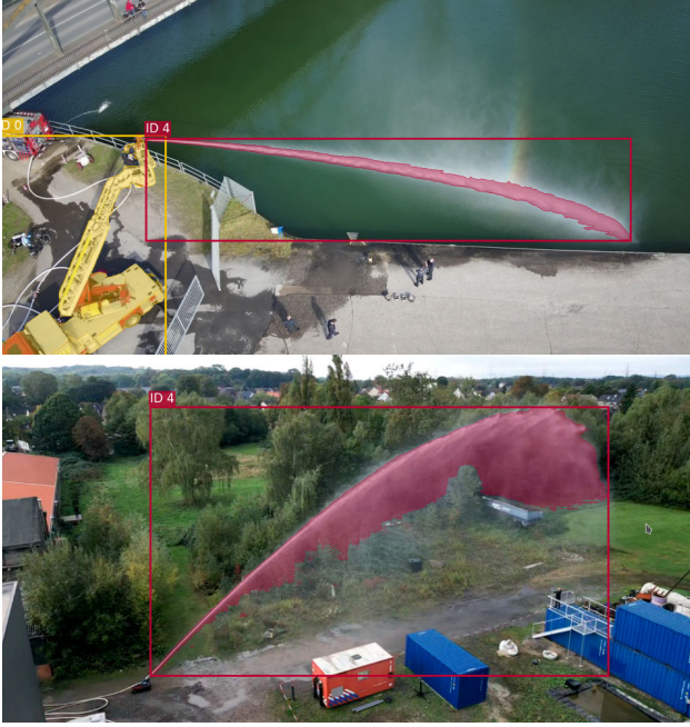
Fig. 8. Detection of the water jet (red). The jet transforms from a coherent jet close to the fire monitor into spray at its end.
