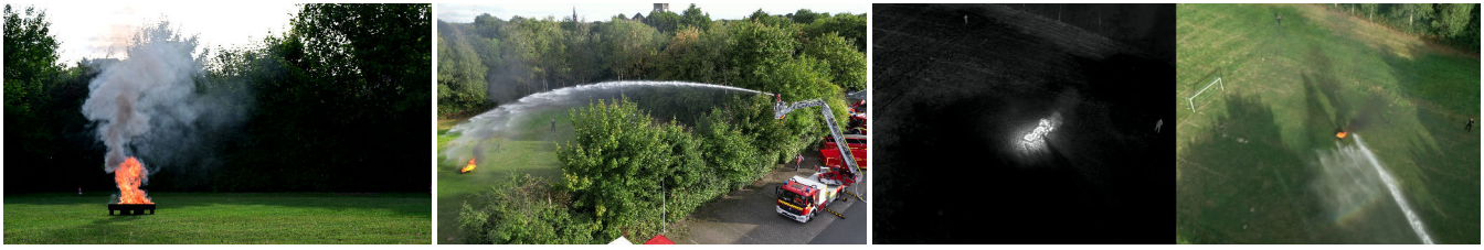
Fig. 9. Integrated system test at a fire station in Dortmund, Germany. The difficult-to-reach fire (left) is hidden behind a tree line, obstructing the view towards the fire from the monitor mounted on a turntable ladder truck. The fire is clearly visible in the UAV footage (right) and enables targeted extinguishing.
