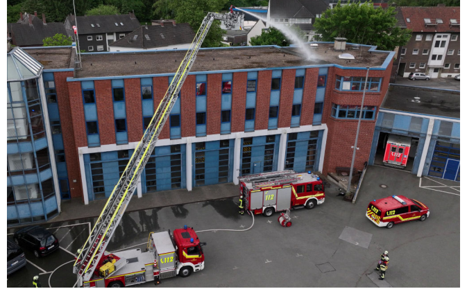
Fig. 1. An automated fire monitor sprays water from an aerial turntable ladder onto a simulated heat source as detected by the UAV.
