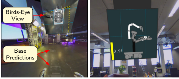
Fig. 17 Locomotion visualizations. Left: Birds-Eye view and predictions of base pose in the future. Right: Side-view for height adjustment.
