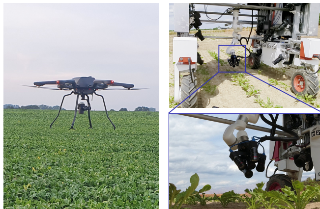
Fig. 1. Left: UAV used to create high-resolution semantic orthophotos in the field. Right: UGV and robotic camera arm setup for crop inspection.
