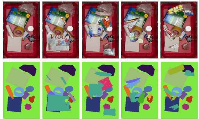
Fig. 6. Generated synthetic scenes. All scenes were generated with the same annotated background frame (left column) for easier comparison. Top row: RGB. Bottom row: Color-coded generated segmentation ground truth.
