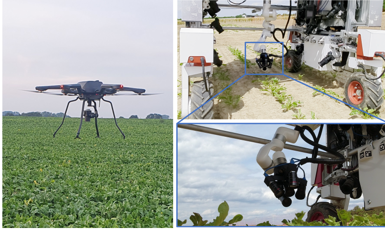
Fig. 1. Left: UAV used to create high-resolution semantic orthophotos in the field. Right: UGV and robotic camera arm setup for crop inspection.
