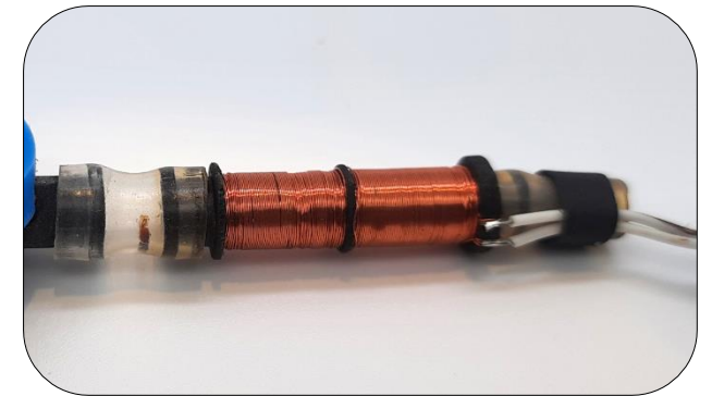
Implemented actuator (without iron armature)
