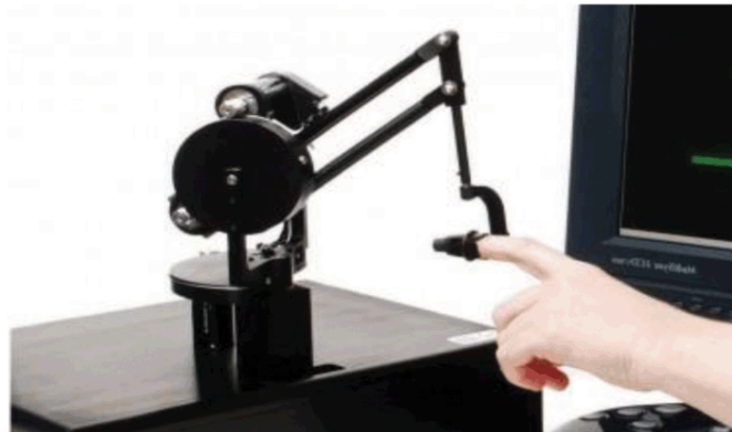
(a) Grounded haptics (e.g., Phantom Premium)
