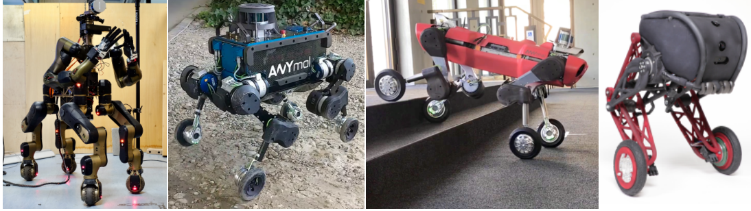
Figure 2.2: Hybrid Robots. From left: CENTAURO (from [13]), Wheeled ANYmal 2018 (from [2]), Wheeled ANYmal 2020 (from [1]), Ascento (from [15])
