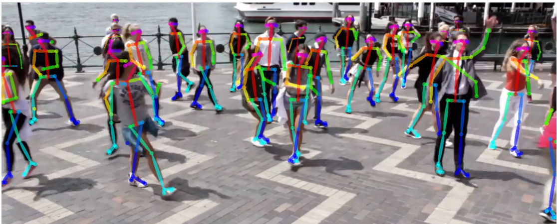
Figure 2.1: 2D human pose estimation for multiple persons simultaneously. Keypoint detections belonging to the same person are linked. [16]
