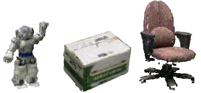
Figure 5: Learned object models at a resolution of 2.5 cm visualized by samples from the color and shape surfel distributions. Left: humanoid, middle: box, right: chair (best viewed in color).
