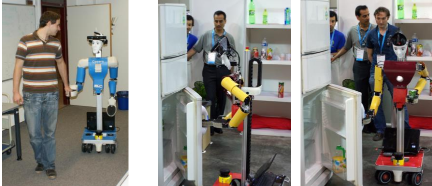
Fig. 3. Left: A person guides Cosero at its hand. Right: Dynamaid opens and closes a refrigerator using compliant control at RoboCup 2010 in Singapore.
