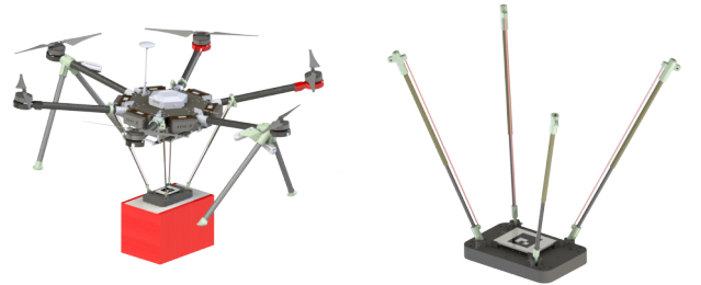
Fig. 9. UAV hardware design. Left: Full assembly. Right: Magnetic gripper with passive compliance. The four telescopic rods are shown in fully extended configuration.
