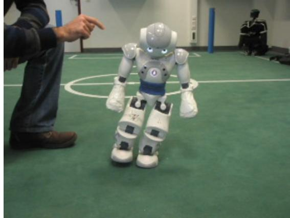
**Fig. 1.** Nao robot reacting to lateral disturbances.
