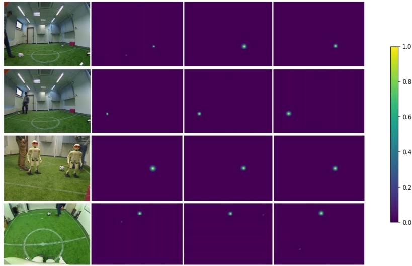
Fig. 8. From left to right: input image, the ground truth, prediction of the neural network, and the final output after post-processing.
