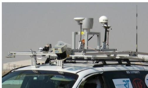
Fig. 1. Left: Velodyne HD Lidar sensor. Right: Placement of the sensor.
