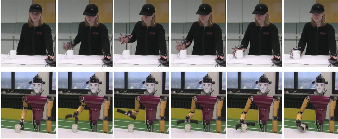
**Figure 1:** The teacher demonstrates a grasping movement (top). From the recorded trajectory, our approach extracts a parameterized motion primitive. The robot imitates the grasp by executing the extracted motion (bottom).
