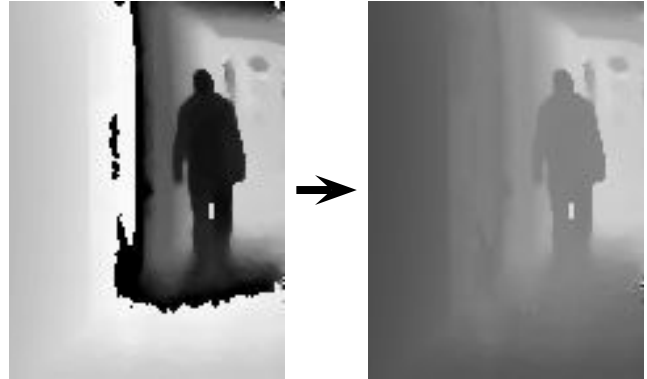
Fig. 1. Unwrapping the input depth image (left). The brightness encodes the measured distance (dark pixels are near, bright pixels far away). The abrupt change from bright to dark in the input image is the phase jump that we want to detect in order to correct the measured distances and to obtain the unwrapped depth image (right).
