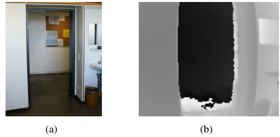
Fig. 2. (a) An image of the scene. (b) Wrapped depth image from the ToF camera. A pixel's gray-scale value corresponds to the measured depth, from dark (close) to bright (far). The dark parts of the image indicate that distance measurements larger than 5 meters are wrapped.
