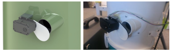
Fig. 3. Bleed actuator for suction regulation. Left: CAD model. Right: Final installation.
