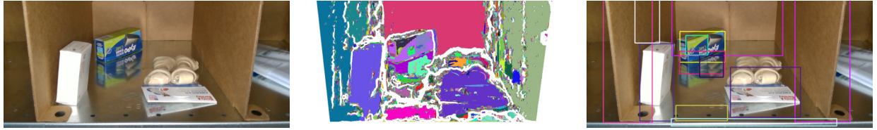
Fig. 6. RGB-D based additional region proposals. Left: RGB frame. Center: Regions labeled using the connected components algorithm. Right: Extracted bounding box proposals.
