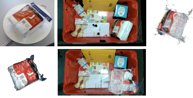
Fig. 8. Pose registration. Left column: Turntable capture, resulting model. Center column: Scene, scene with initializations. Right column: Final registered model.
