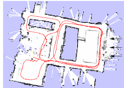
Fig. 5. Grid map learned from data obtained by a human carrying a laser range finder in the hand. The arrows indicate parts of the environment in which the sensor perceived mainly invalid observations. The estimated trajectory is shown in red.
