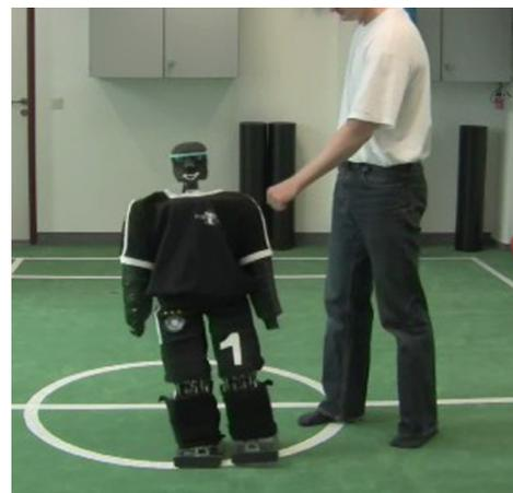
Fig. 1. Our robot Dynaped rejects lateral disturbances with capture steps.
