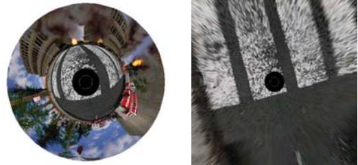
(a) Omnidirectional image (b) A bird-eye view projection data obtained from the of Fig. 1a. simulation environment.
