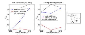
Fig. 10. Evaluation with real humanoid robot Jupp: Walking forward against a wall at various angles. Left: results at low speed, mid: results at high speed, right: experiment configuration.
