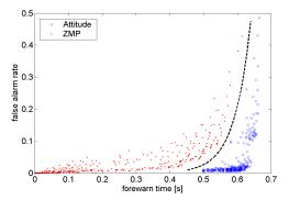
Fig. 8. Detection comparison of the attitude sensor instability indicator and the ZMP criterion: forewarn time and false alarm rate depending on detection parameters. The dashed line shows a clear separation of both instability indicators.
