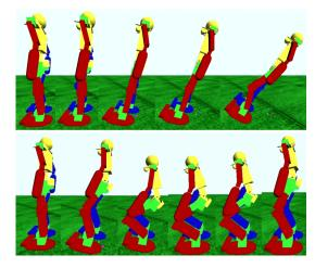
Fig. 7. Robot disturbed by an impulse force on its chest while walking backward at speed (0, -0.3, 0). The upper picture shows the robot falling when no stabilizing reflex is activated. In the lower picture the stop walk reflex has been activated. The robot stops walking, crouches down and thereby prevents the fall.
