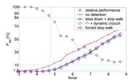
Fig. 9. Fall probability when disturbing the robot during walking by an impulse force without any reaction, with slow down and stop walk reactions, with dynamic crouch and with forced stop walk actiovation of 96ms before the disturbance. The dotted line shows the relative performance. The 10% working point is marked by the dashed lines.
