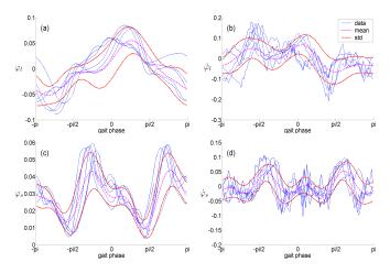
Fig. 3. Attitude sensor data of six gait cycles vs. gait phase  $\Theta$  at speed (0,0.5,0) with means and standard deviations obtained by inverse Fourier transform of the model: (a) lateral tilt, (b) derivative of lateral tilt, (c) sagittal tilt, (d) derivative of sagittal tilt.
