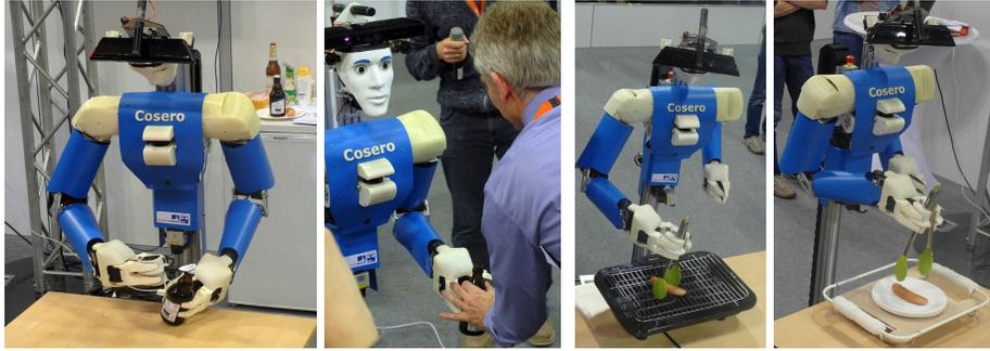
**Fig. 6.** Tool use demonstrated in the RoboCup German Open 2014 final: Opening a bottle and picking a sausage from the BBQ.
