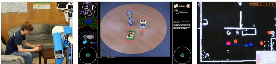
**Fig. 7.** Handheld teleoperation interface based on a tablet [16] (left). The user can e.g. select the object to grasp (center). Estimated locations of tagged objects (right).
