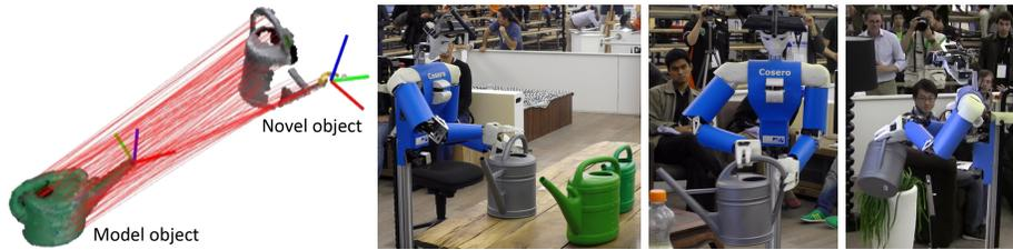
**Fig. 5.** Manipulation skill transfer demonstrated at RoboCup 2013 in Eindhoven: watering a plant with an unknown can based on non-rigid registration of a can model to the novel can [13].
