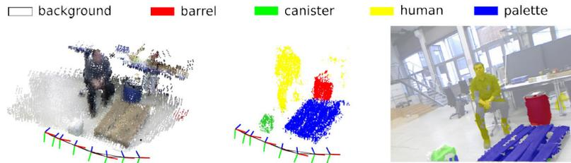
**Fig. 4.** Semantic mapping from a moving RGB-D camera [8].
