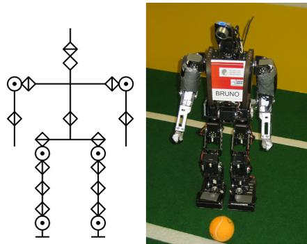
Fig. 1. Left: Kinematic structure of the robots. Right: Humanoid Robot Bruno (DD2008 model).
