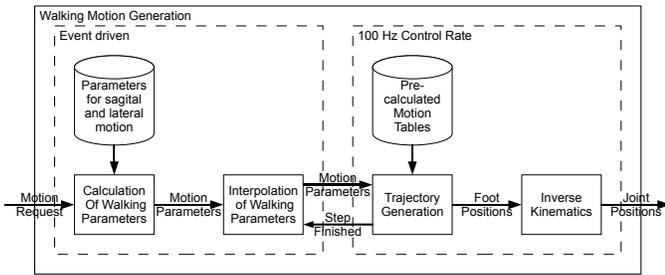
Fig. 4. Structure of the open loop walking motion generation.
